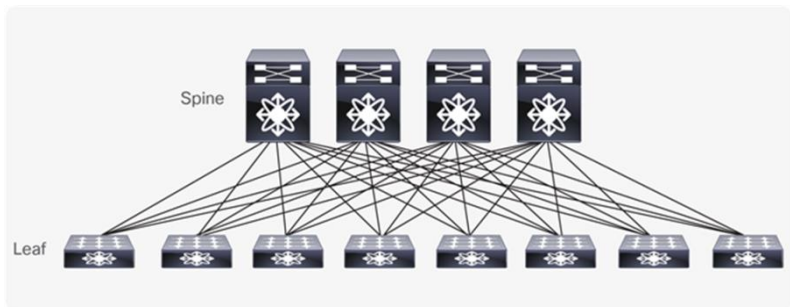
Gambar 8.9: Spine and leaf topology (Cisco, 2020)
