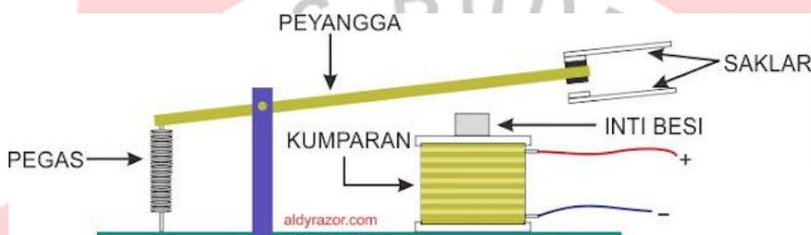
**Gambar 2.5 Cara Kerja Relay Arduino**
