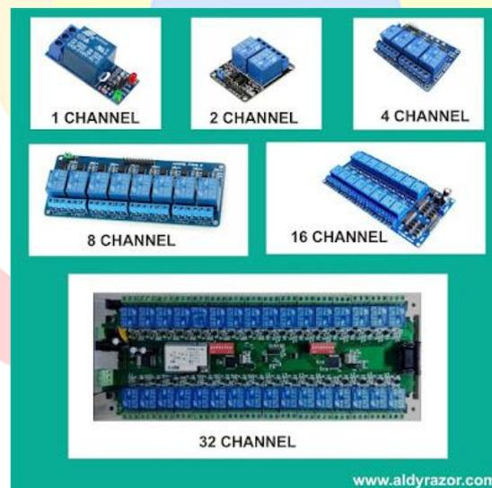
**Gambar 2.4** Macam-macam Relay Arduino
